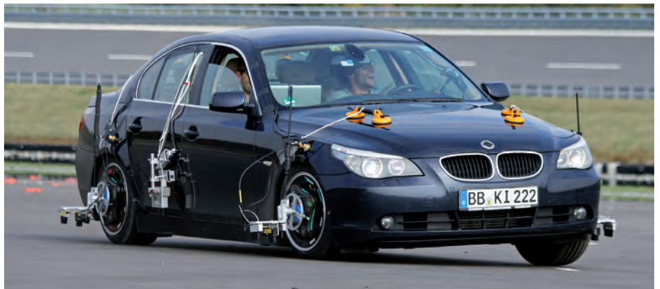
The RoaDyn P1HT wheel torque transducer with optimum handling for tractive resistance measurements
