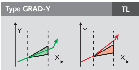
Evaluates the gradient dY/dX between two vertical lines
